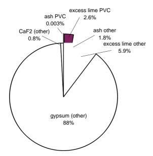
Figure 5 Allocation to PVC in the filtercake: less then 3 wt%. (Configuration B: Wet scrubber with effluent evaporation).
