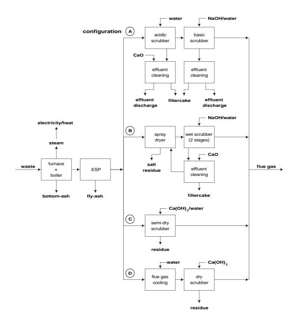
Figure 3 Typical flue gas cleaning configurations.
