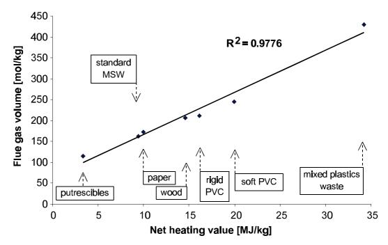
Figure 11 Flue gas volume versus net calorific value.
