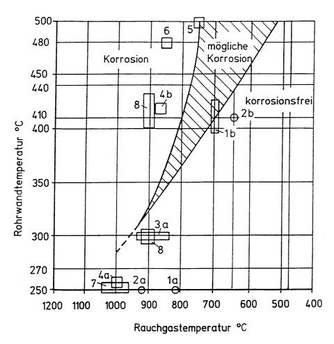
Figure 2 Probability of corrosion depending on the temperature [Born,1997]. Numbers refer to specific MSWC facilities:
