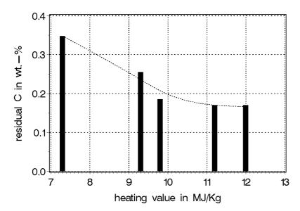
Figure 1 Residual carbon in bottom-ash versus heating value of the feed (combustion temperature 1050 °C) [Vehlow,1996b].
