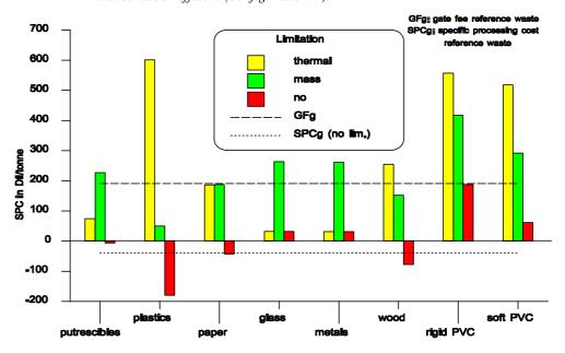
Figure 10 Specific processing costs for a MSWC facility with **evaporation** of the purified wet scrubber effluent (configuration B).
