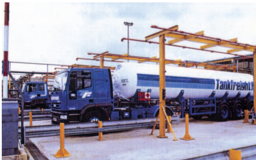
Fig.3.6. Road Tanker with Vinyl Chloride labelled according to UK regulations
