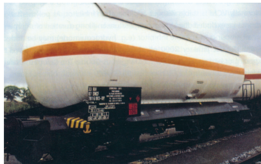
Fig. 3-2 Rail tanker for Vinyl Chloride stabilized
