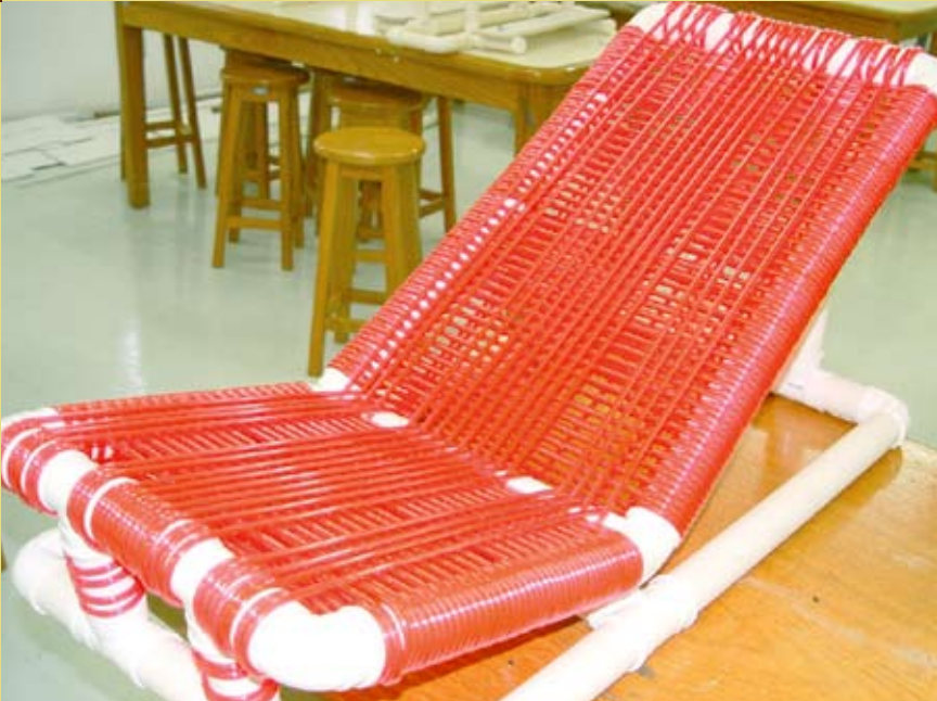
Reclining chair made of lightweight PVC pipes with flexible fabric. Young patients can easily be lifted into the bathtub with it.
